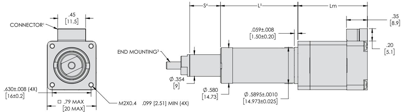
1. S6B-ZR(LF)(SN) connector shown. Wire harness with JST ZHR-6 mating connector and flying leads included with motor. For wiring diagram and connector details, see page 46.
