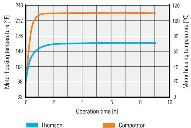
The curves were generated with a 1.5 A / 2.33 V, 1.8° NEMA 17 single stack, rotating screw stepper motor. Test ran with a 0.9°, 24 VDC chopper drive and a 4-2516 lead screw at an ambient temperature of 20 °C.
