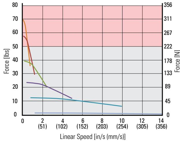
Note: All motor load curves were generated with a 40 VDC, 2-phase ON driver and full stepped at the motor rated current. They account only for motor performance - different nut and motor combinations may yield different performance characteristics. Performance plots for other lead screw and motor winding configurations can be generated at [www.thomsonlinear.com/smla](http://www.thomsonlinear.com/smla).
