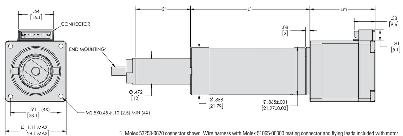
1. Molex 53253-0670 connector shown. Wire harness with Molex 51065-06000 mating connector and flying leads included with motor. For wiring diagram and connector details, see page 46.
