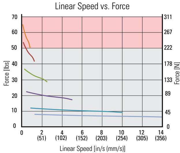
Note: All motor load curves were generated with a 40 VDC, 2-phase ON driver and full stepped at the motor rated current. They account only for motor performance - different nut and motor combinations may yield different performance characteristics. Performance plots for other lead screw and motor winding configurations can be generated at [www.thomsonlinear.com/smla](http://www.thomsonlinear.com/smla).
