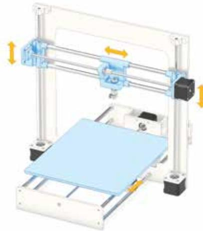
Utilizing a stepper motor linear actuator on a 3D printer can eliminate the need for couplings, bearings and supports while increasing stroke length and print volume.
