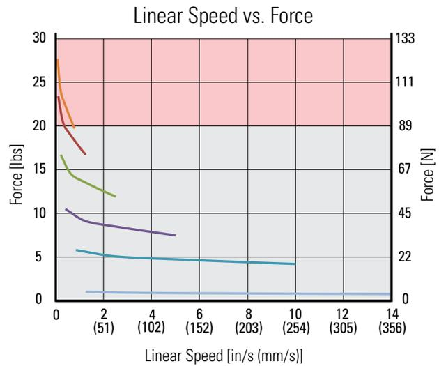
Note: All motor load curves were generated with a 40 VDC, 2-phase ON driver and full stepped at the motor rated current. They account only for motor performance - different nut and motor combinations may yield different performance characteristics. Performance plots for other lead screw and motor winding configurations can be generated at [www.thomsonlinear.com/smla](http://www.thomsonlinear.com/smla).
