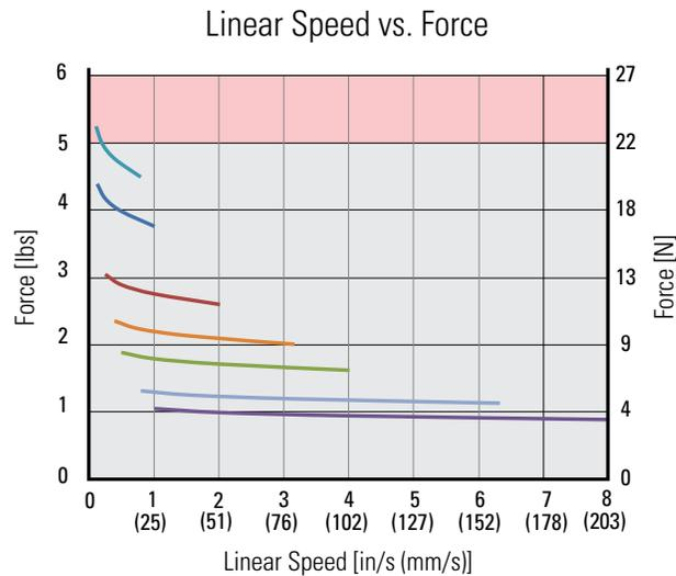
NOTE: Motor load curves were generated with a 24 VDC, 2-phase ON driver and half stepped at the motor rated current. They account only for motor performance - different nut and motor combinations may yield different performance characteristics. Performance plots for other lead screw and motor winding configurations can be generated at [www.thomsonlinear.com/smla](http://www.thomsonlinear.com/smla).
