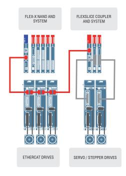
EtherCAT slave nodes are connected via the Flexslice EBUS and the EtherCAT connector (lower RJ45 socket). Up to 64 axes are supported using CSP, CSV and CST modes of operation. Total slave connections can be up to 128 nodes including I/O and complex devices.
