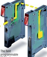
rne field programmable FPGA allows customisation of the functionality of some Flexslice Modules using *Motion* Perfect. The program can be "locked-down" creating a unique function for a machine builder which protects the functionality from being copied.
