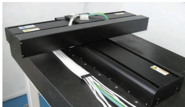
In this case, the bottom axis carries the work piece in one direction and the top axis carries the end effector to move in the orthogonal direction.
