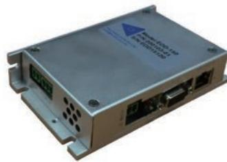
A two position electronic drive, EOD from Akribis can be used to drive the voice coil motor in the manner described above. The peak current, peak current duration and holding current can be adjusted to control the start of motion and the holding force of the voice coil at stationary position.
