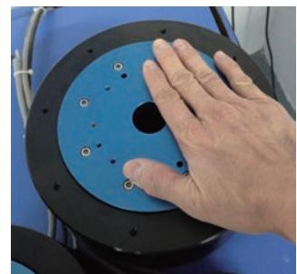
Rotate motor by hand to feel cogging effect
