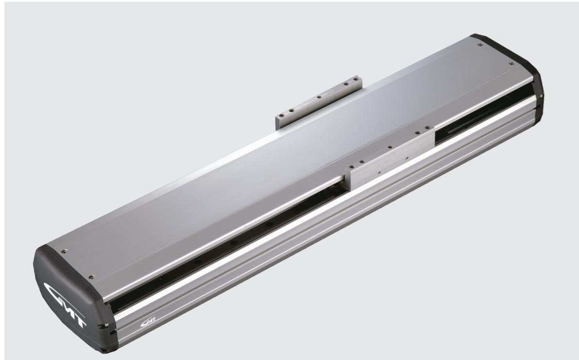
Maximum Stroke 1250 mm    Maximum Speed 2000 mm/s    Motor Output 400W    Ball Screw Ø20 mm    Linear Guide 20X15-2 Pc
