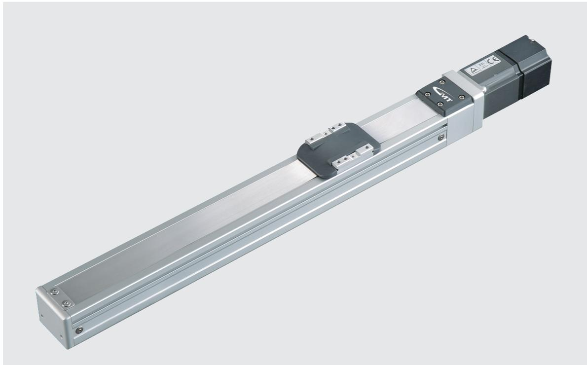
Maximum Stroke 800 mm    Maximum Speed 500 mm/s    Motor Output 100W    Ball Screw Ø12 mm    Linear Guide 24X8.5-1Pc
