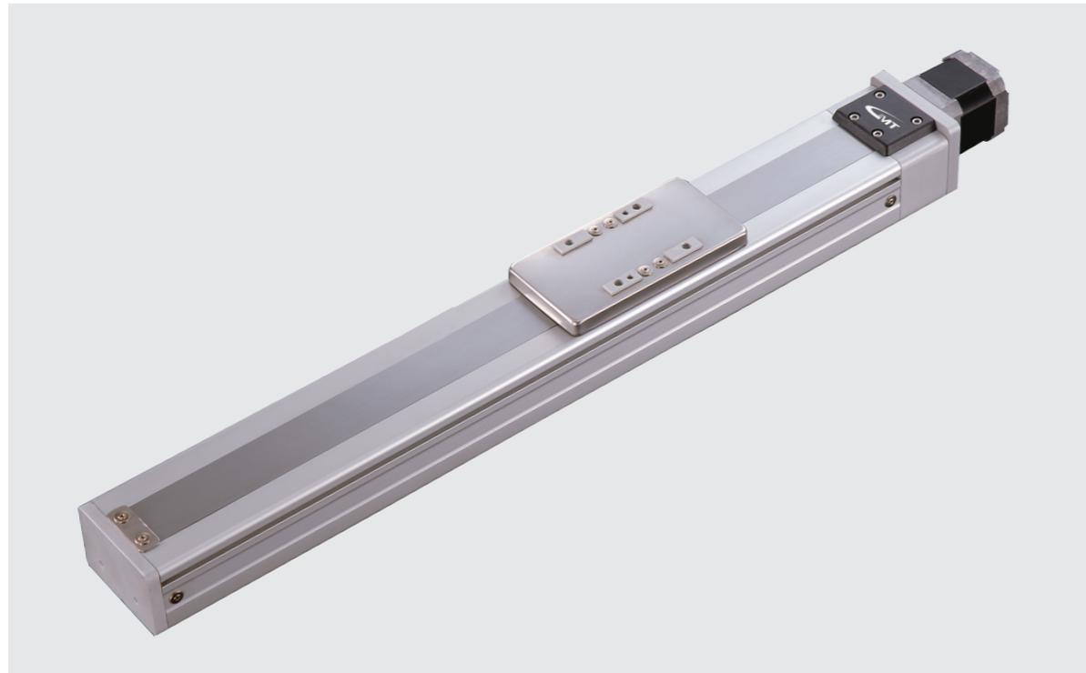
Maximum Stroke 800 mm    Maximum Speed 83 mm/s    Motor Output 57    Ball Screw Ø12mm    Linear Guide 9.5X42-1Pc
