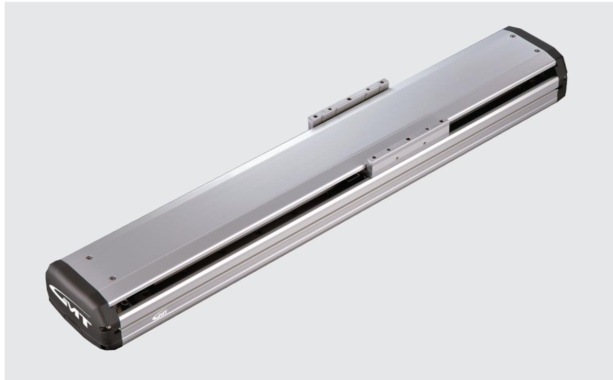
Maximum Stroke 1050 mm    Maximum Speed 1000 mm/s    Motor Output 400W    Ball Screw Ø16 mm    Linear Guide 15X12.5-2 Pc
