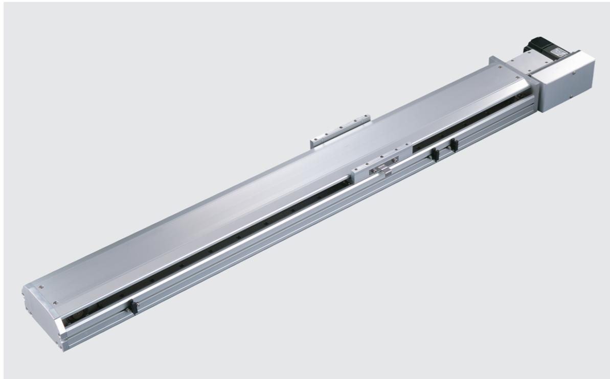
Maximum Stroke 3050 mm    Maximum Speed 2000 mm/s    Motor Output 200W    Belt Width 22 mm    Linear Guide 15X12.5-2 Pc
