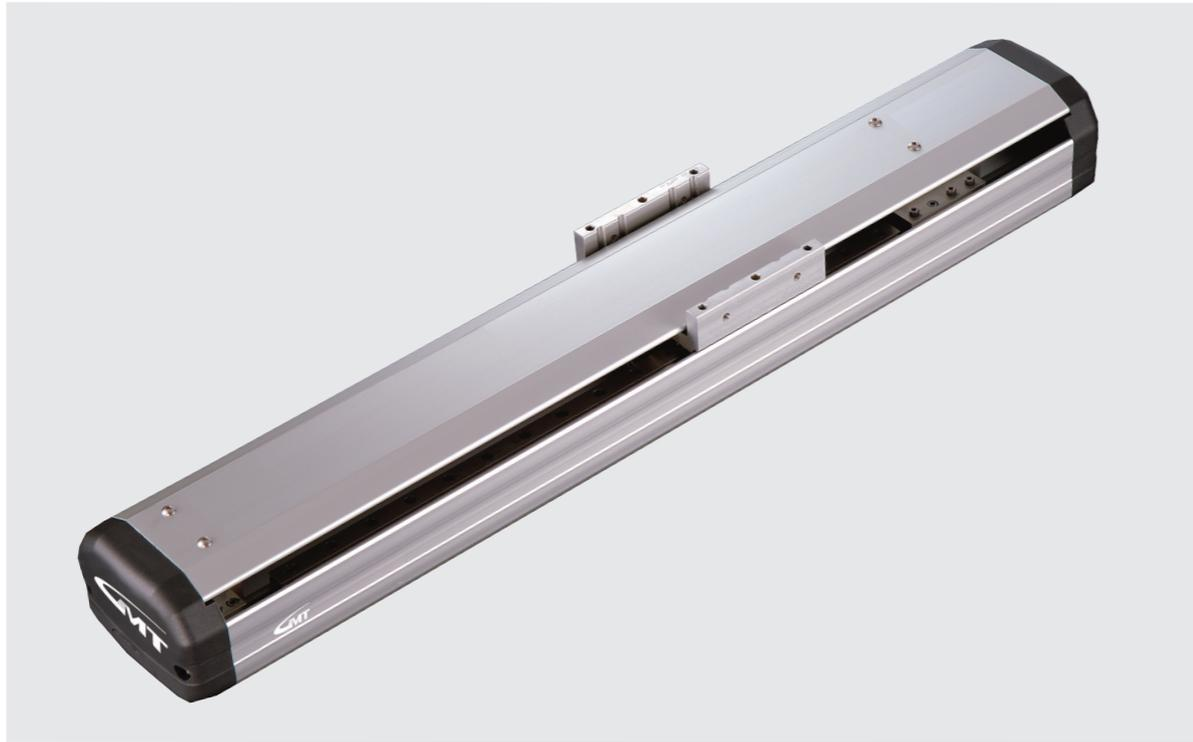
Maximum Stroke 1050 mm    Maximum Speed 1000 mm/s    Motor Output 100W    Ball Screw Ø16 mm    Linear Guide 12X7.5-2 Pc
